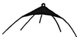
Figure 6. In the parachute spinnaker a broad strip of wood or light metal replaces the small wooden headboard
