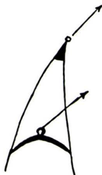
Figure 7. Spinnaker, showing two hauling parts for reducing the size for very light breezes
