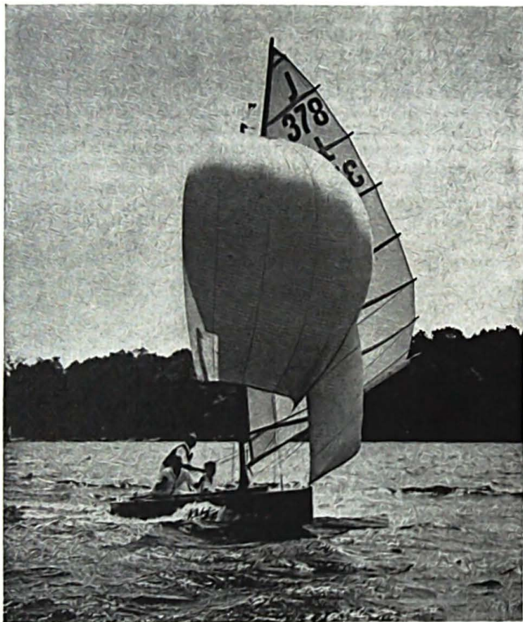
Right. A parachute spinnaker on a 20-Square-Metre racer. It is effectively spilling the wind into a light, overlapping jib
