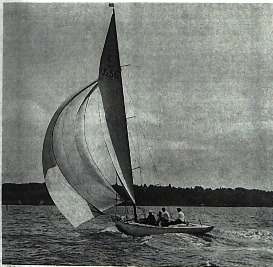
The American challenger "Jill," winner of the Seawanhaka Cup on the Clyde. She is using a double or balloon spinnaker as a balloon jib, a new departure which proved markedly effective. In fact this sail was used with the apparent wind slightly forward of the beam
