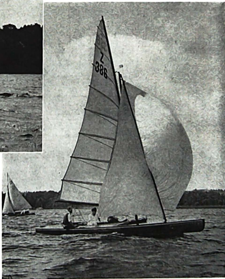
Left. A parachute spinnaker which solves the problem of getting a large sail with the short spinnaker booms prescribed by the rules where the base of the fore triangle is short
