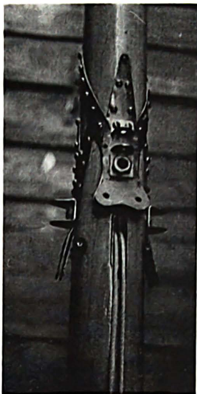
Mast tangs and spreader fittings on a six-meter's mast. These are carefully calculated to carry a load equal to the breaking strength of the wire
