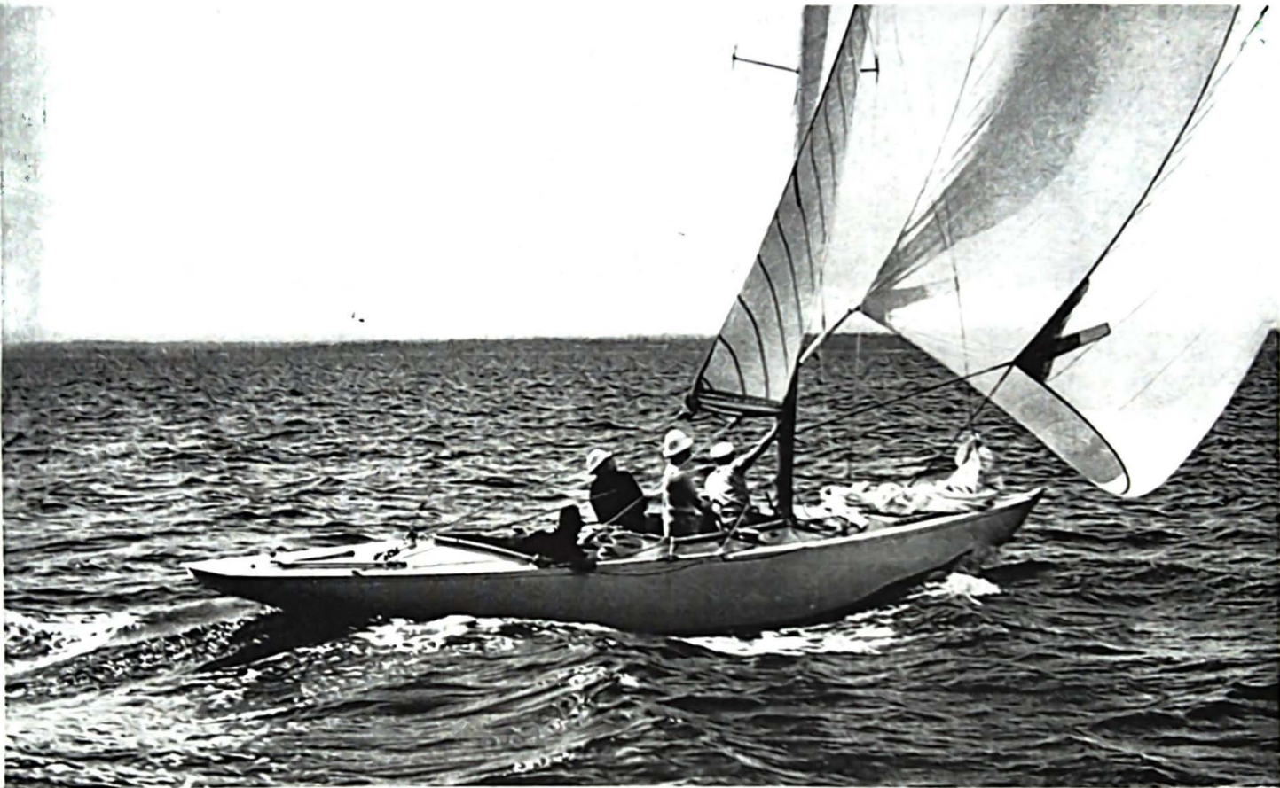
The Six-Metre "Djinn" has geared winches operated from under the deck, the winches alongside the main cockpit having large drums for Genoa sheet and spinnaker gear. Note the Genoa sheet lead blocks on the rail, the boom downhaul and the rod rigging
